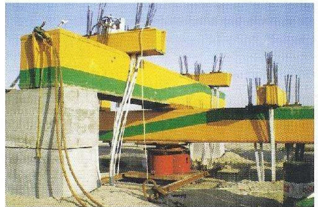
TENSION STATIC LOAD TEST SETUP
